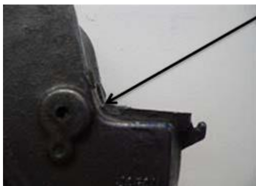
Photo 3: Steering bracket with the turning stop removed
