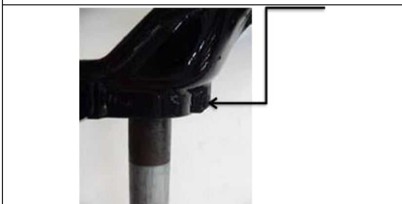
Photo 2: Steering bracket with centre turning lug removed
