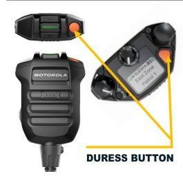
The Duress function on the GWN radios provide enhanced safety for SLSQ Members. When activated, it triggers both a visual and audible alert, serving as an emergency beacon that notifies SurfCom through their internal systems.
