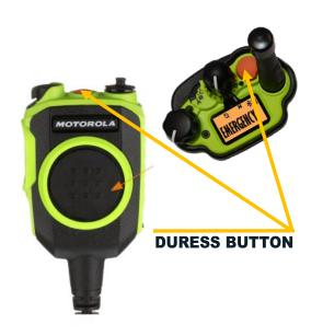
The Duress function on the GWN radios provide enhanced safety for SLSQ Members. When activated, it triggers both a visual and audible alert, serving as an emergency beacon that notifies SurfCom through their internal systems.
